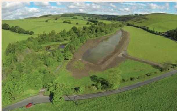
Figure A1.11 Kitson Mill flood storage pond (courtesy Tweed Forum)
