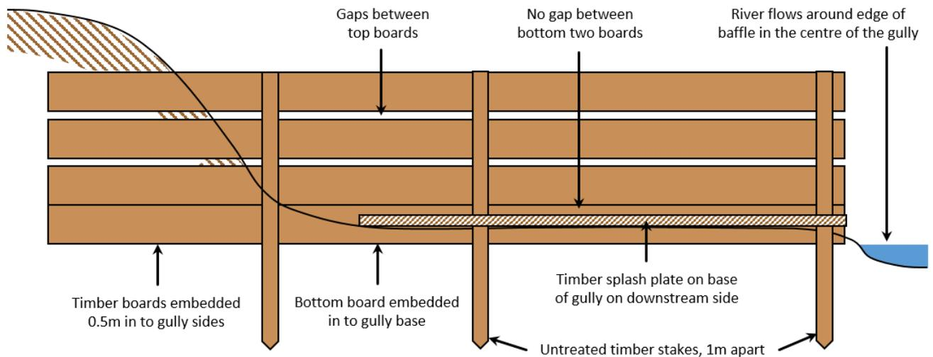
**Figure 3.8 | A timber baffle.** An example of a timber baffle. Diagram adapted from Moors for the Future.
