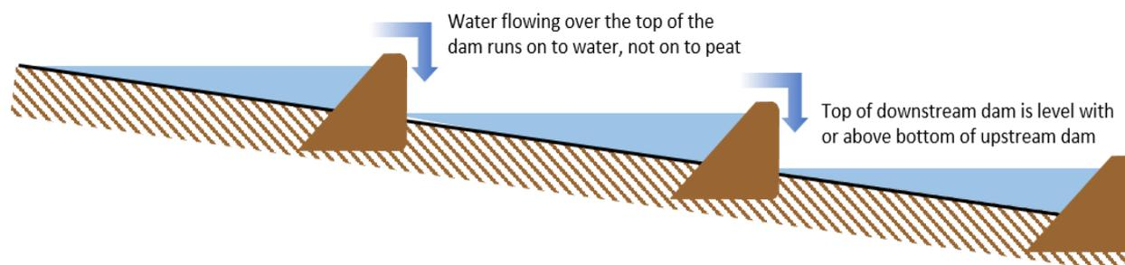
**Figure 3.4 | Optimal spacing of dams.** Dams should be installed using a 'top-to-toe' principle to avoid undercutting and erosion. On average, dams should be placed every 7-12m, depending on slope, and water should fill the entire section between dams. Pictures adapted from Moors for the Future Partnership fact sheets.
