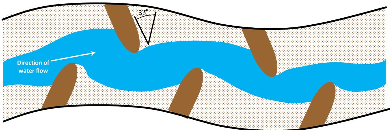
**Figure 3.6 | Baffle placements down a large gully.** Optimum placement will be to avoid bank erosion, thus keeping the main water flow in the centre of the gully and away from the re-profiled edges.
