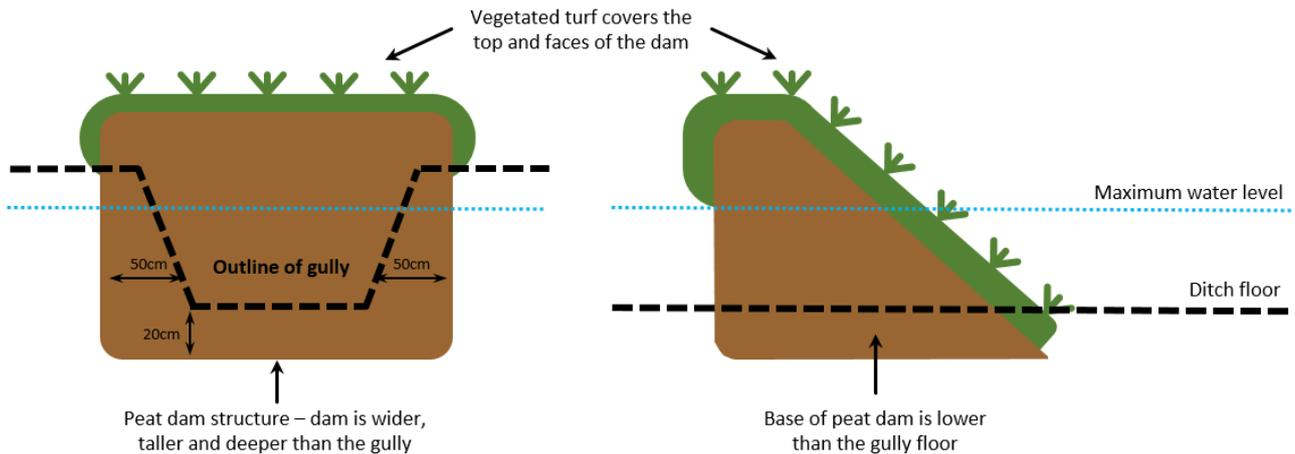
**Figure 3.1 | The construction of a peat dam.** Showing the front view (left) and the side view (right) of peat dam construction. The vertical edge of the dam is on the downstream side of the dam. Pictures adapted from Moors for the Future Partnership fact sheets.
